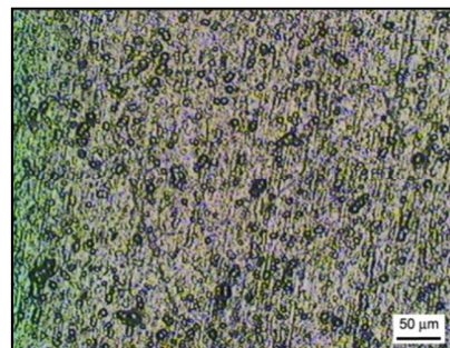
Fig. 2: OM images of the AA6061 after etching treatment.
