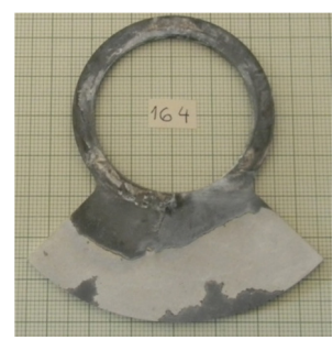
Fig.13d. Coupon after Period III at FACIRI (level -15m).
